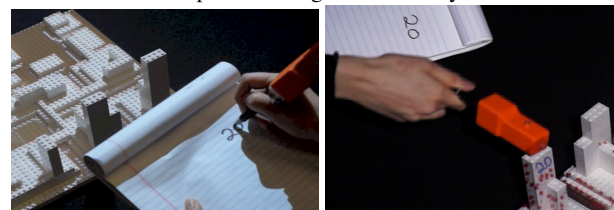
Figure 2. Tapping the pen on co-located physical objects allows for augmented annotation of the physical model with real-time written content.
