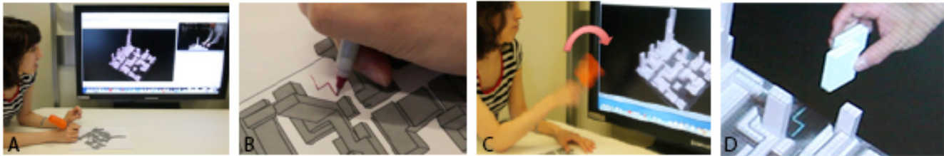
Figure 1. Augmented remote reality, leveraging familiar design tools such as pen, paper and prototyping building blocks. (A) The physical prototype is manipulated by a remote collaborator, with whom a designer communicates through a videoconference. (B) The pen gesture-based Augmented Participatory Design system captures sketches. (C) Flicking the pen towards the model on the screen instantly transfers the paper sketch to the corresponding spot on the remote model, with which the remote collaborator creates new physical prototypes (D).
